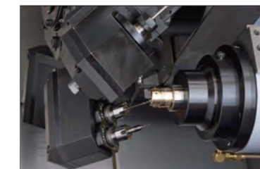
variation 01 | Skewed Hole Drilling
