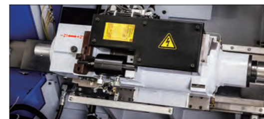
Main Spindle | The headstock stroke of 350mm
