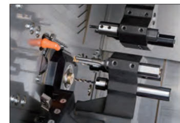
variation 01 | Machining and Positioning of the Twin Turrets
