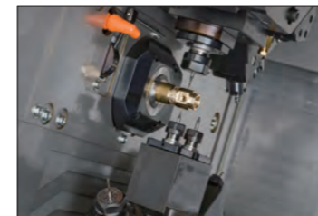
variation 02 | Cross Drilling+Cross Milling
